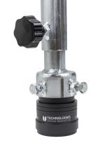
Snap Connector in the sensor cup
