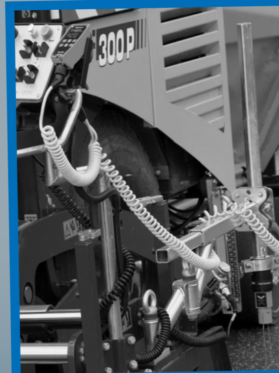
Mini-Line® HS301 Grade Control Kit with G221
