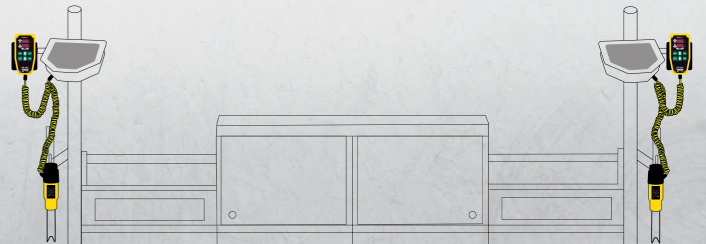
HS301 Double Grade Control Kit with G221 Single-Sonic sensors as set up on the asphalt paver. Sensor and controller connect to the 10-pin plug of the asphalt paver with a V-Cable in each side of the screed.
