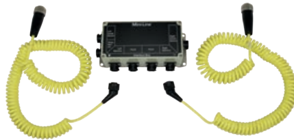
Connect two coiled cables to the Interfacebox with 6-pin bayonet connectors. Connect the other end of the cables to the 10-pin plug on the machine.
