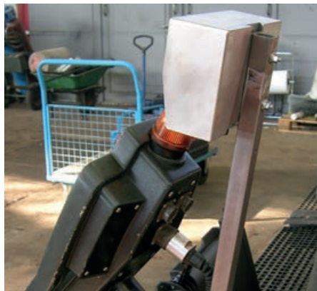
Figure 19 - Example of mounting of Control Box by mounting a square metal tube on the side plate of the screed.
