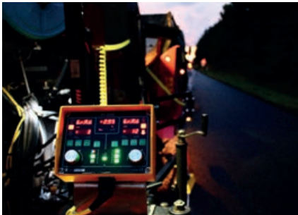
The PL2005 automatically adjusts the brightness of the LED display for bright or dark surroundings.
